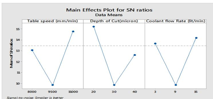
**Fig. 3 Main effect Plot for SN Ratio**
