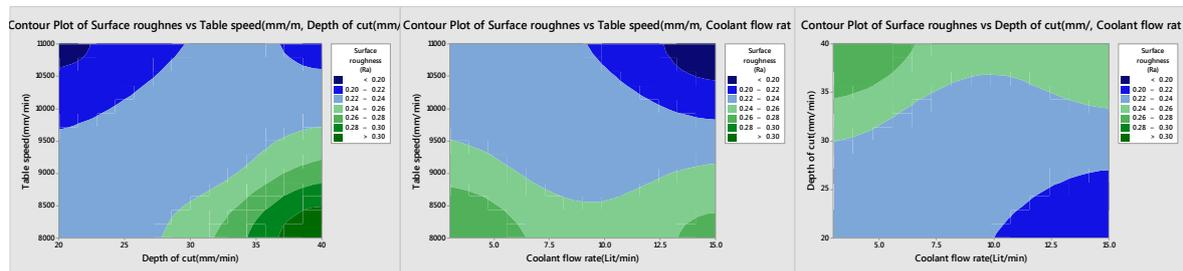
Fig. 7:-Conture plot (a) Surface roughness Vs table speed and depth of cut (b) surface roughness Vs table speed and coolant flow rate (c) surface roughness Vs depth of cut and coolant flow rate.
