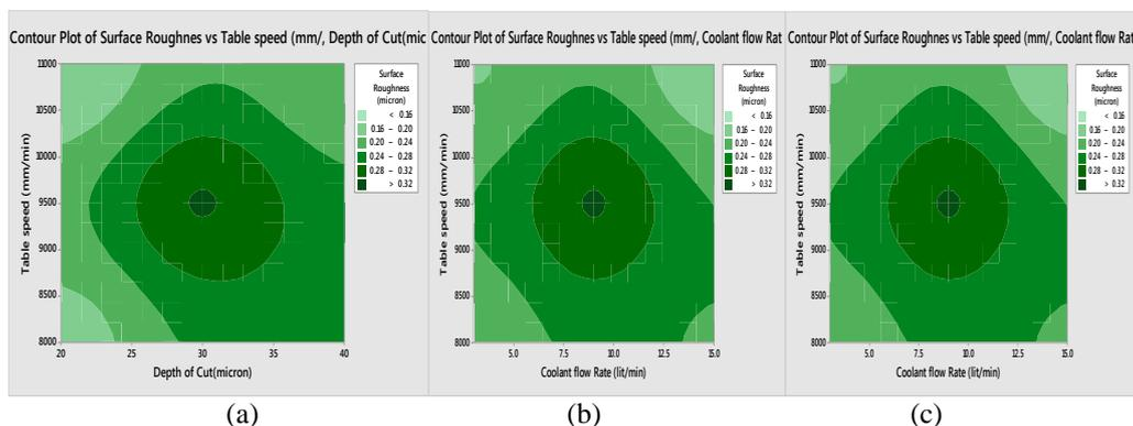
Fig.4 :-Conture Plot (a)Surface roughness Vs Table speed and depth of cut (b) Surface roughness Vs table speed and coolant flow rate (c) Surface roughness Vs depth of cut and coolant flow rate.
