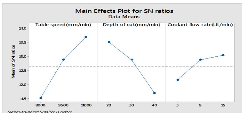
Fig. 5 Main effect plot for SN ratio
